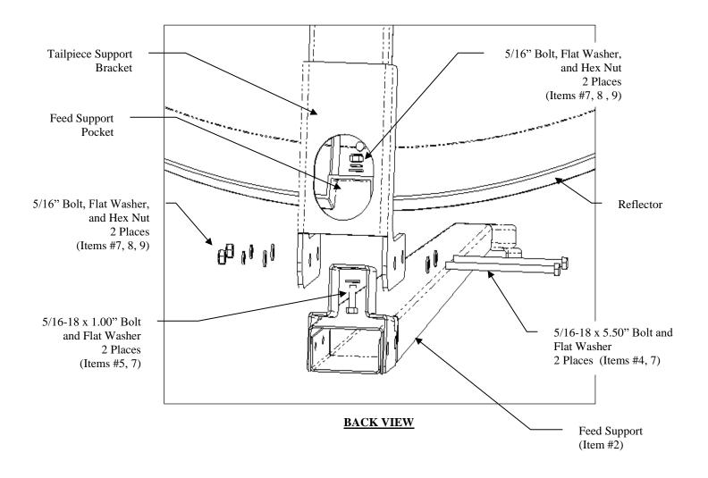
4. Attach a feed rod to the mounting hole in the side of the reflector with a 5/16-18 x 1.00-inch bolt and flat washer (Items #5, 7) and secure with a flat washer, lock washer, and hex nut (Items #7, 8, 9) on the back side of the reflector.
